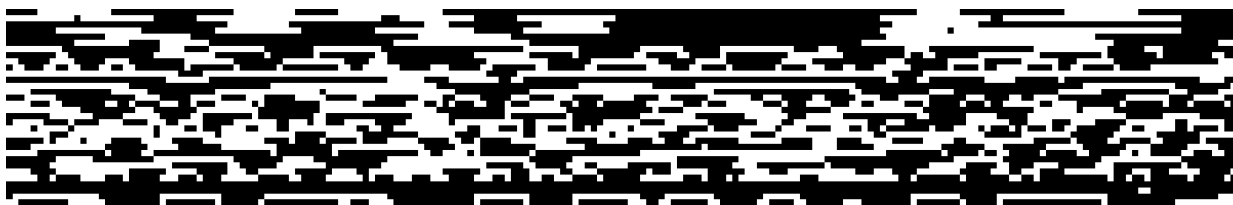
Figure 3.4 A graphical representation of the Chromaprint for the first 10 seconds of “Ziggy Stardust”, by David Bowie. Each vertical block represents a 32 bit integer, with 1 encoded as black and 0 as white.
